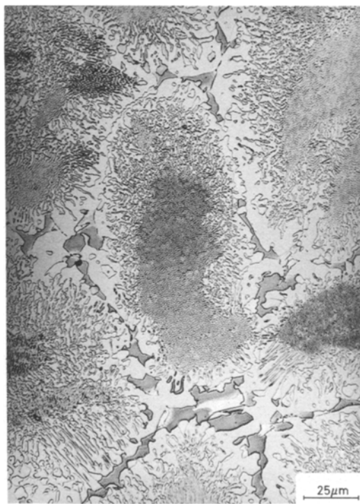
Figure 2 Optical micrograph of the transverse section of a Co-Sm-Sn eutectic alloy directionally solidified at 100 \mu\text{m sec}^{-1} .
